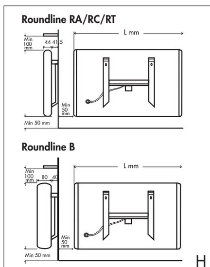
Make sure the distance between the end of the radiator and the nearest wall is at least 50 mm. The distance from the radiator to a possible window-sill should be at least 100 mm (**Picture H**).
